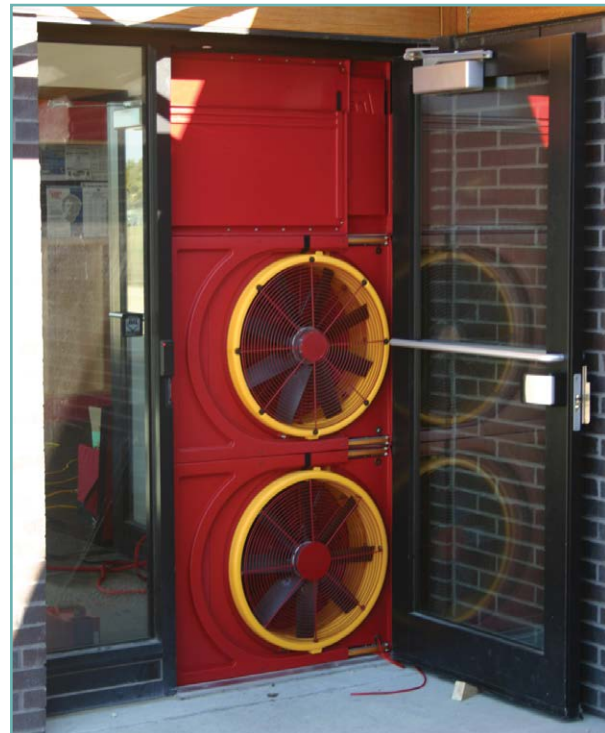
Figure 4-5 Blower door installation with two blowers; this would be suitable for most small to medium-sized MURBs
